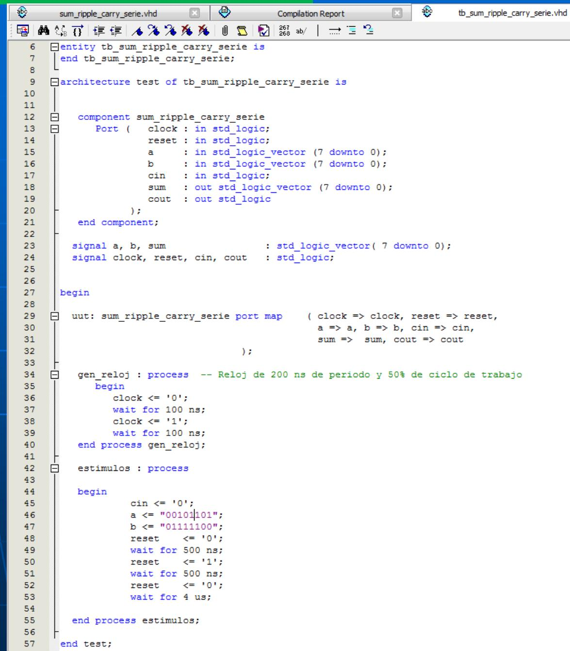
The screenshot shows a VHDL testbench for a ripple-carry adder. The code is as follows:
