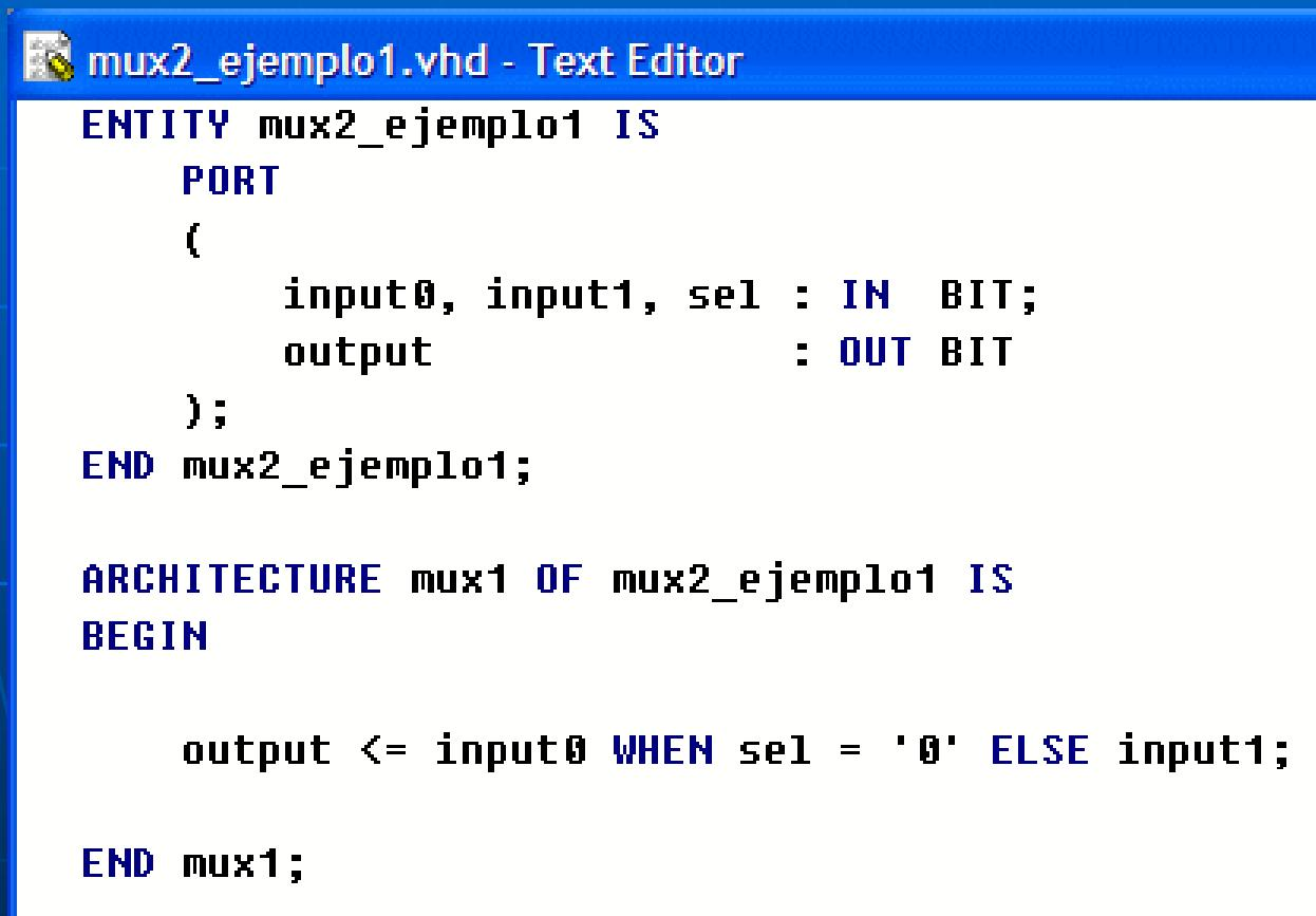
The screenshot shows a text editor window titled "mux2\_ejemplo1.vhd - Text Editor". The code is written in VHDL and defines a 2:1 multiplexer. It starts with the ENTITY declaration, followed by the ARCHITECTURE section which contains a WHEN-ELSE statement to select between two inputs based on the control signal 'sel'.
